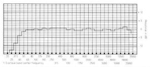
Frequency response of the 4313B taken with  $\frac{1}{3}$ -octave band pink noise. Measured response contour of a typical system averaged through an inclusive arc of 120° in the horizontal plane does not deviate more than 3 dB from the above curve.
