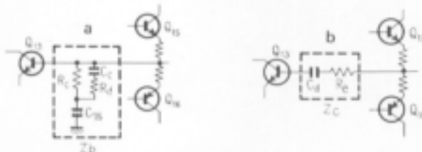
Fig. 9 Equivalent Circuit of Treble Boost and Cut
