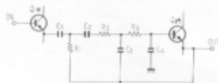
Fig. 7 Circuit Diagram of Filter Circuit
