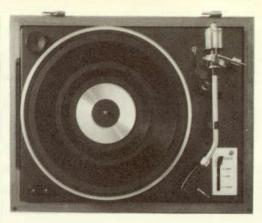
EXPENSIVE HEAD SHELL PROVIDED: The SR-1050C is supplied with an expensive head shell made of a special light alloy. Large holes are punched in its top surface to make it as light (8 grams) as possible; its edge is specially bent to serve as a reinforcement rib for added strength; and the part that couples to the cartridge is doubly constructed to avoid resonance. Its gold-plated connection terminals are fashioned as a plug meeting EIA standards, an be coupled to tonearms of other makes.
